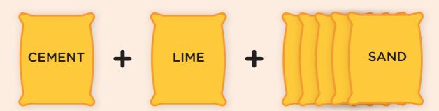
Mixtures are sometimes also expressed as a percentage. In this instance, the mortar mix would be rounded up to 15% cement, 15% lime and 70% sand.
