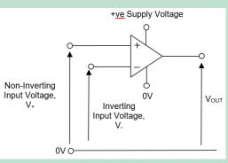
The operation of the comparator is such that it amplifies any difference between the two input voltages by a very large amount, causing the output to be at one of the extremes of the power supply connected to it. This means that the output voltage will be either high or low and can only fall into one of the following categories.
