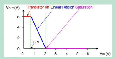
There are **three** key parts to this graph, which is known as the transistor voltage transfer characteristic:
