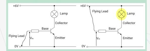
A **small** base current is used to control a much *larger* current in the collector circuit.
