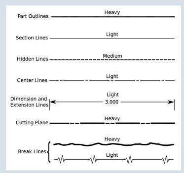
Line weights in engineering drawings also follow British standards and should again be used in traditional and CAD work.
