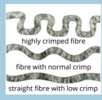
Wool fibres have a natural crimp which traps air, making wool a good insulator. The tighter the crimp, the warmer the wool. The scales on it also trap air.
