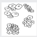
Linen's smooth surface gives it a slight lustre, whilst the hollow centre of the fibres allow for good absorption.
