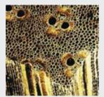
The micro-holes in bamboo fibres allow good absorption. It is anti-microbial and prevents the growth of bacteria.
