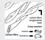
The hollow cavity in the cotton fibre allows for absorption. The twist in the smooth fibre adds strength.
