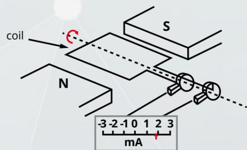
To generate a **larger** current, you can use a coil with **more turns**, use **stronger magnets** or a coil with a **larger area**. Turning the coil **faster** will also increase the current but will make the **frequency** of the current increase too.
