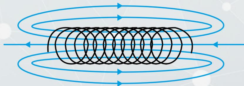
A larger current will create a stronger field, more turns on the coil will create a stronger field but changing the direction of the current will reverse the direction of the field.
