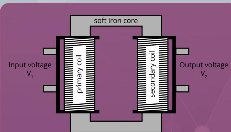
The coil with the most coils will have the higher voltage. e.g. In a step-up transformer the **secondary coil will have the most turns** to increase the voltage.
