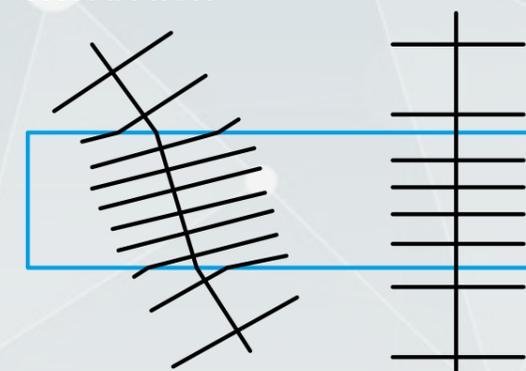
Notice the change in direction and the change in wavelength due to the change in speed.
