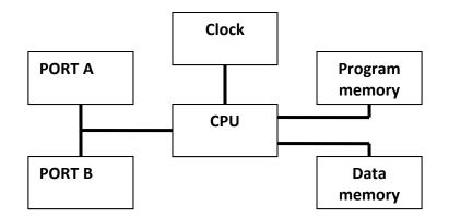
The **CPU**: Central Processing Unit performs the programme operations and controls data flow.
