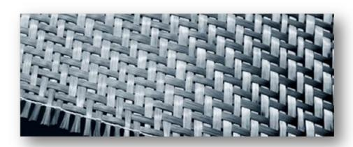
The binding polymer is often a thermoset resin such as epoxy, but other thermoset or thermoplastic polymers, such as polyester or nylon are sometimes used.
