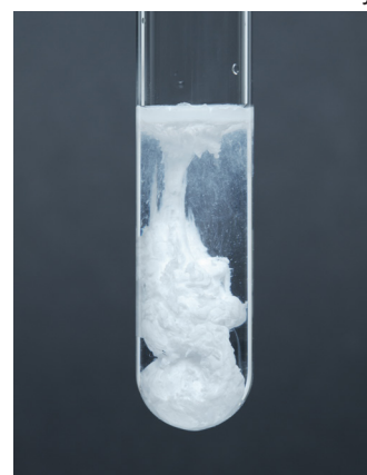
Prawf am ïon clorid GIPhotoSctock / Science Photo Library
