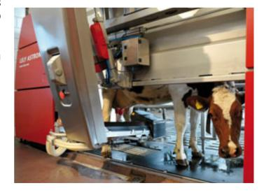
The milking machines connect automatically to the cow's teats and turn off when the milking is complete. A safety mechanism ensures that cows can only be milked for a certain number of times per day, with some cows choosing to be milked four or five times a day.
